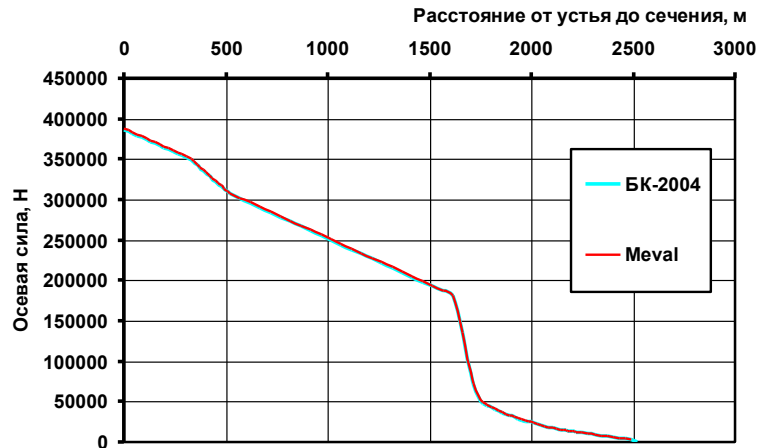
Figure 1. Results of calculation of axial forces during lifting BC from a borehole with a horizontal end
